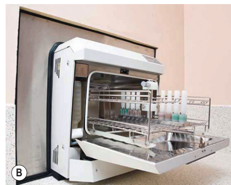
Fig. 37.4 (A) A diagram showing the instrument decontamination cycle. (B) A washer disinfector (a glorified washing machine with a disinfection cycle). (Part (A) from the Health Technical Memorandum 01-05 – Decontamination in primary care dental practices UK 2009, with permission; Crown Copyright.)
