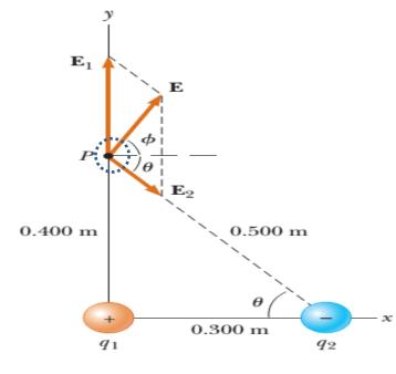
$$E_1 = k_e \frac{|q_1|}{r_1^2} = (8.99 \times 10^9 \,\text{N} \cdot \text{m}^2/\text{C}^2) \frac{(7.00 \times 10^{-6} \,\text{C})}{(0.400 \,\text{m})^2}$$
