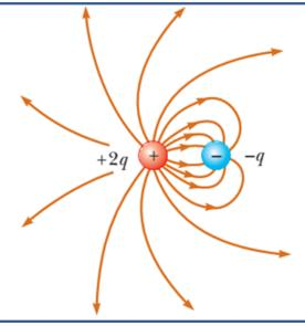
The electric field lines for a point charge of **2q** and a second point charge of **q**.
